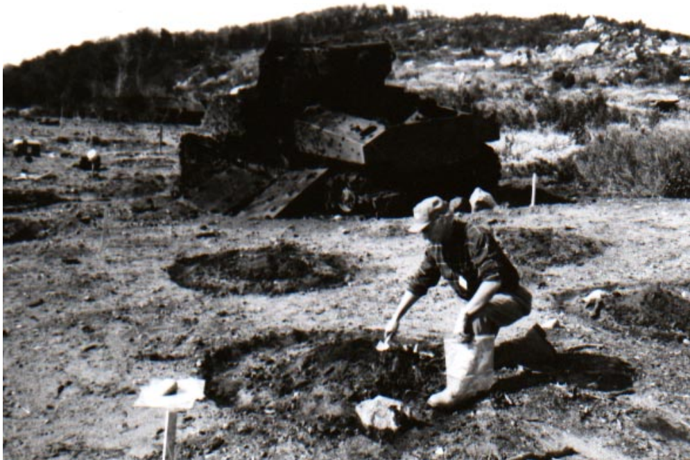
Figure 7. Subgrid sampling path and sample collection.
