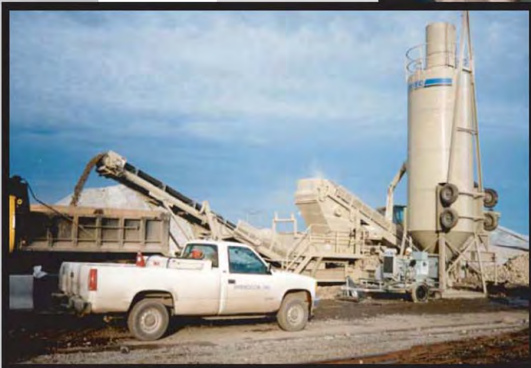
A Pugmill Mixing Contaminated Soil with Fly Ash to Reduce Total Leachable Lead Concentrations
