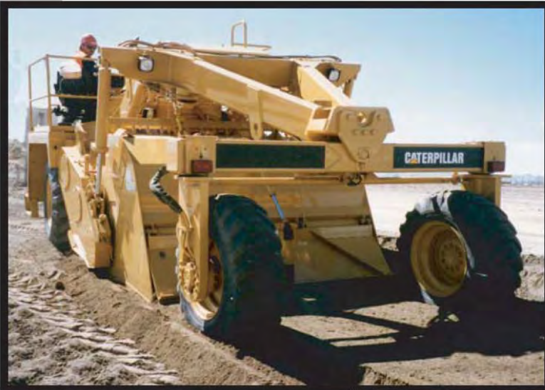
Soil Stabilizer Used to Mix Reagents for Stabilization
