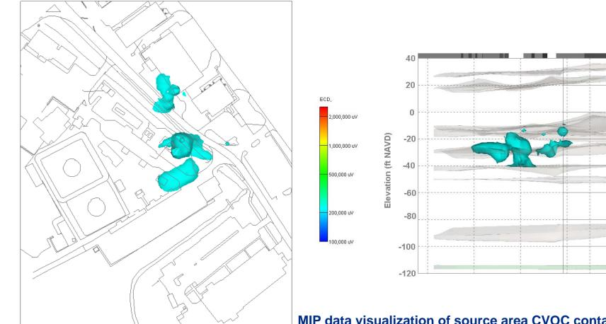
MIP data visualization of source area CVOC contamination identified (prior to this investigation through to be only between two buildings).
