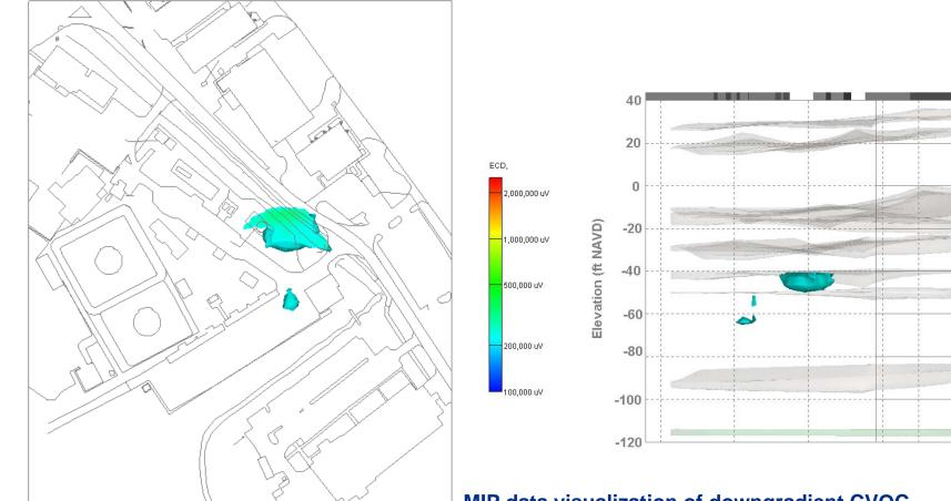
MIP data visualization of downgradient CVOC contamination (prior to this investigation was thought to be more isolated).
