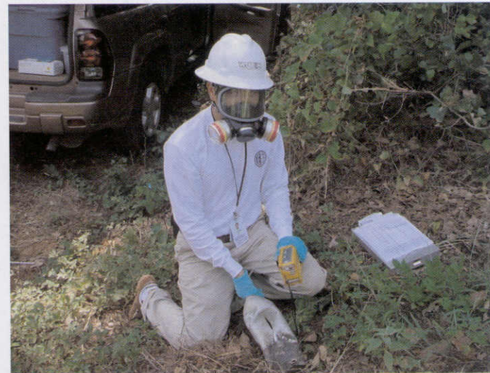
A Weston Solutions employee performs an air-monitoring evaluation on a piece of debris from the space shuttle Columbia. (Photos courtesy Weston Solutions, Inc.)
