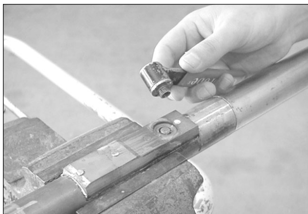
Figure 6.1 Unthread the membrane from the probe block.
